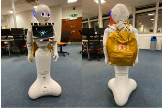
Fig. 4. Overall outfit of our system, including a Pepper robot, a ReSpeaker USB Mic Array and two OAK-D Camera attached on a wood frame, and a Raspberry Pi 4 stored in a bag
