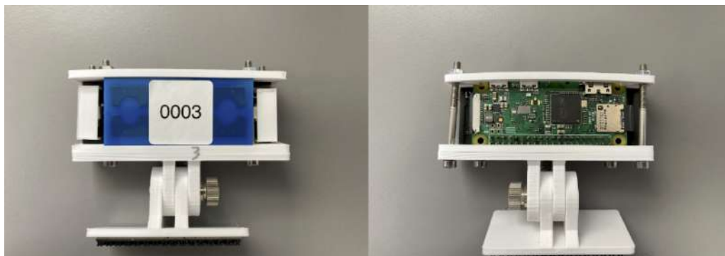
Figure 3.1: A radar node in an adjustable mount. (left) A X4M05 radar mounted at the front. (right) A Raspberry Pi Zero W mounted at the rear.
